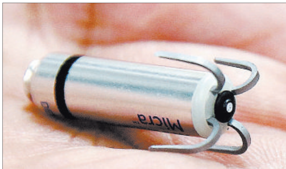
The Medtronic miniature pacemaker was approved by the FDA last year. Instead of surgery, the tiny device can be inserted by a catheter through an artery to the heart. When it wears out in 12 years, another can be inserted without the removal of the first.
